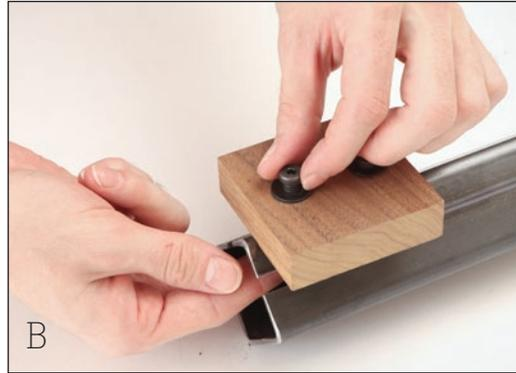
A and B: Align the mounting block and thread the bolt (with washer) into the threaded rivets at the top of the leg.
